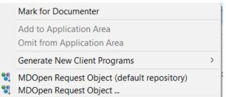
3. select MDOpen Request Object (default repository) if the check-out should occur for the instance of MDCMS that is marked the default within the MDOpen Repository view
